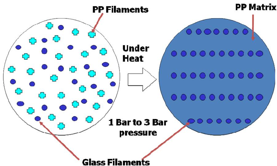
Figure 1. Construction of a bundle of fibres
