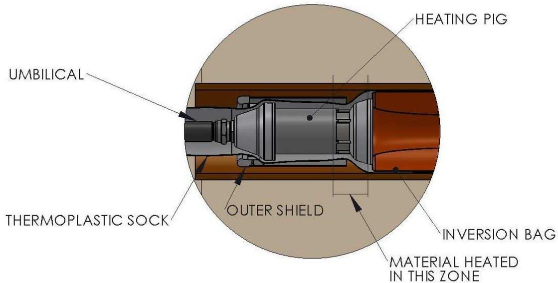
**Figure 3. – Detail of Heating Pig Inside the Composite Sock**
