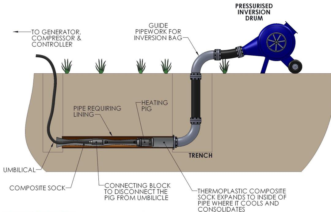
Figure 2. – Schematic of the Aqualiner process
